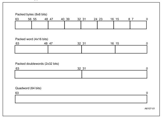
The MMX instructions move the packed data types (packed bytes, packed words or packed doublewords) and the quadword data type to-and-from memory or to-and-from the Intel architecture general-purpose registers in 64-bit blocks. However, when performing arithmetic or logical operations on the packed data types, the MMX instructions operate in parallel on the individual bytes, words or doublewords contained in a 64-bit MMX register.
